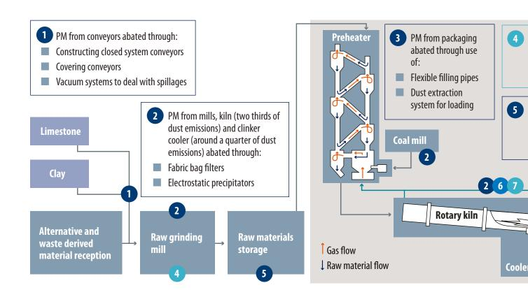
Figure 7: The cement manufacturing process and the emission of NOx, PM and SO, and their abatement
