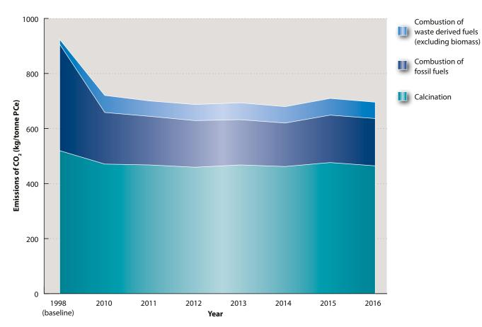
Figure 10: Reduction in direct emissions of CO, in 1998 (base year) and 2010-2016
