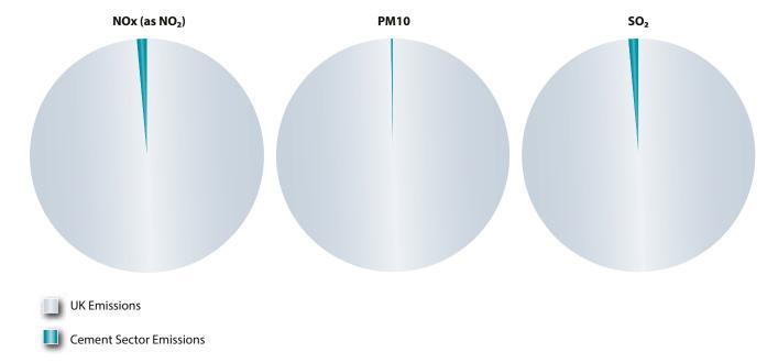
Figure 3: Proportion of UK emissions of NOx, PM10 (PM with particle size less than 10 micrometres) and  $SO_2$  arising from cement manufacture [Source: National Air Emissions Inventory]
