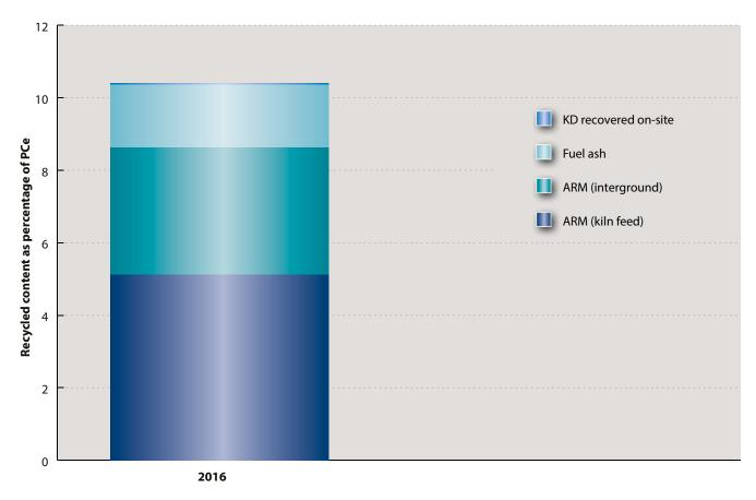
Figure 8: The total recycled content of UK produced cement from kiln dust (KD) recovered on site, fuel ash recycled as mineral content, alternative raw materials (ARM) interground with clinker to produce cement and ARM fed to the kiln (kiln feed)
